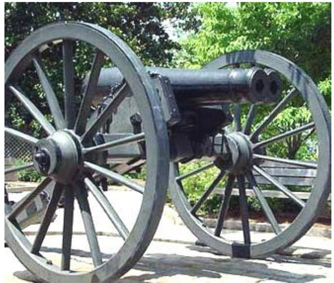
Even though the ignition is in the middle, if one ignited a nanosecond before the other, the result of two joined cannon balls would be catastrophic. One ball would exit the barrel slightly ahead of the other, thus wrapping back around. There is no way to ignite both barrels simultaneously with two primers.
